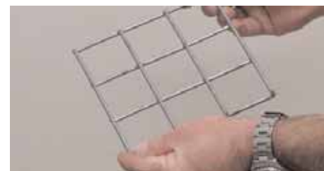
galvanized 2" x 2" x 8.5 gauge welded wire
