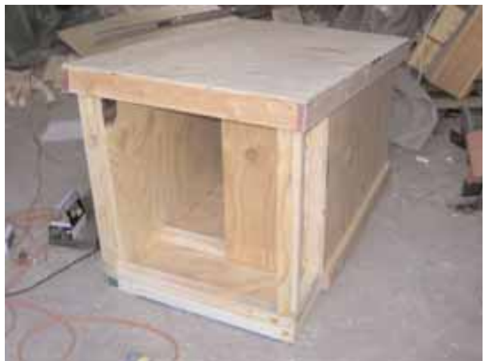
Summer configuration of bungalow. The plywood front baffle can be removed and stored under the roof.
