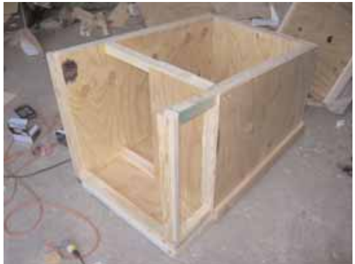
Assembled bungalow with roof and front baffle removed.
