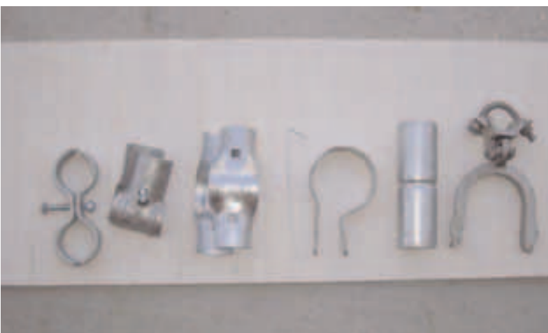
12. Corner post hardware: rail end band around it, attached to the rail end at the end of the top rail. It is used to attach top, middle and bottom horizontal rails to the big corner and door posts.
