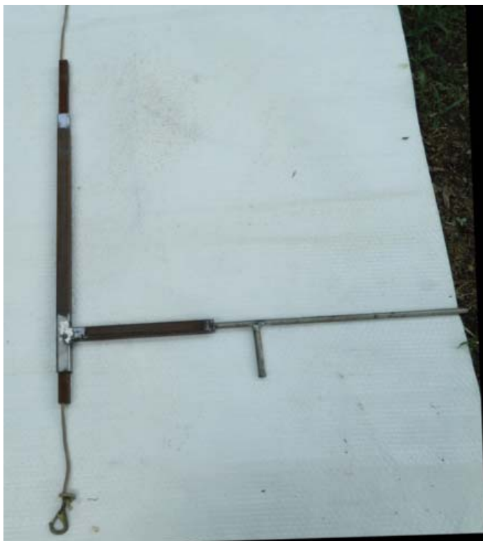
Assembled interlock with shift gate partly up, main gate bolt is blocked.
