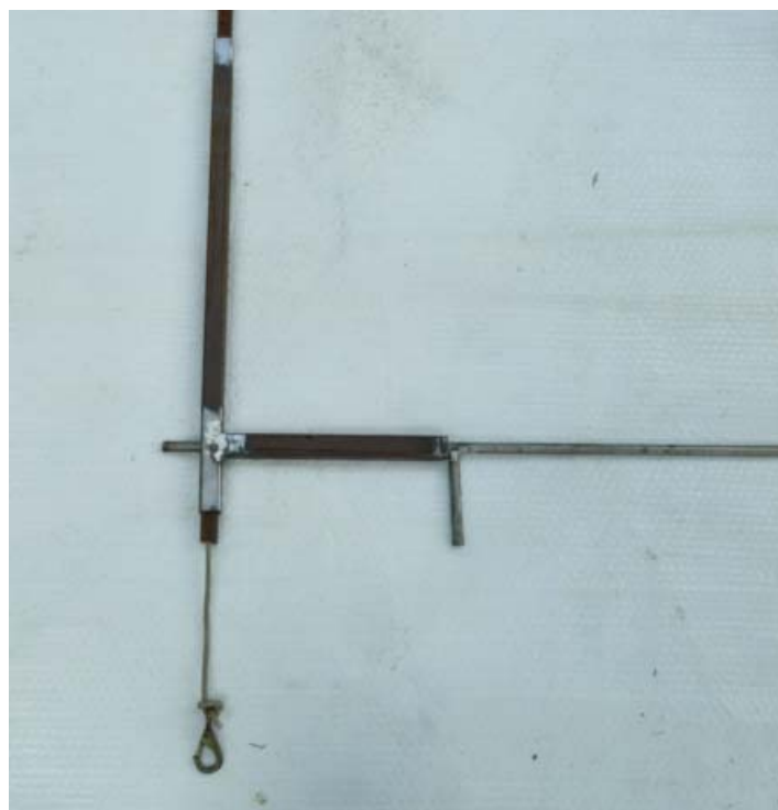
Assembled interlock with main gate unlocked, protruding bolt shows shift gate is closed.
