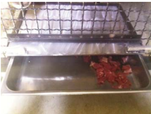
Pan being put in feed slot. Lid stays in place while tray slides inside slot.
