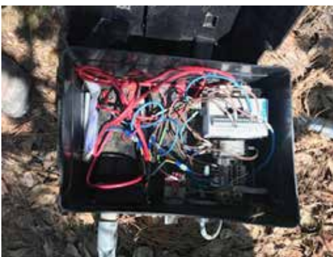
This is the inside of the gigasensor: all of the components are able to fit into this hard plastic box, making it easily portable.
